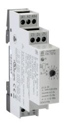
Dold on-delay relay timer, 0.05 to 120 seconds selectable timing range, 24 VAC/VDC and 110-127 VAC operating voltage, 2A contact rating, (1) SPDT timed relay output(s), 35mm DIN rail mount, screw terminal(s).
