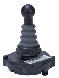
Schmersal selector switch, IP65, IP67, IP69 and IP69K, 22mm, 4-position, momentary, (4) N.O. contact(s), plastic base, plastic bezel, Operator: gray, joystick, 25mm, round, plastic.
