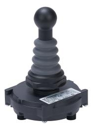
Schmersal selector switch, IP65, IP67, IP69 and IP69K, 22mm, 2-position, momentary, (4) N.O. contact(s), plastic base, plastic bezel, Operator: gray, joystick, 25mm, round, plastic.
