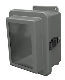
Stahlin RJW series enclosure, NEMA 1/3R/4X/6P/12, 8 x 6 x 6in (HxWxD), wall mount, fiberglass reinforced polyester, gray, raised single-door, (1) quick-release latch, padlock hasp and staple, SAR acrylic window.
