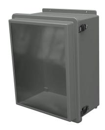
Stahlin RJW series enclosure, NEMA 1/3R/4X/6P/12,  $20 \times 16 \times 10$  in (HxWxD), wall mount, fiberglass reinforced polyester, gray, raised single-door, (2) quick-release latches, padlock hasp and staple, SAR acrylic window.
