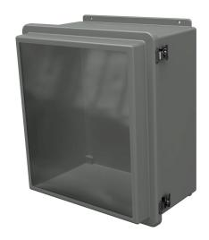
Stahlin RJW series enclosure, NEMA 1/3R/4X/6P/12, 18 x 16 x 10in (HxWxD), wall mount, fiberglass reinforced polyester, gray, raised single-door, (2) twist-lock latches, SAR acrylic window.
