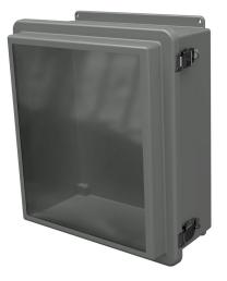
Stahlin RJW series enclosure, NEMA 1/3R/4X/6P/12, 16 x 14 x 7in (HxWxD), wall mount, fiberglass reinforced polyester, gray, raised single-door, (2) quick-release latches, padlock hasp and staple, SAR acrylic window.
