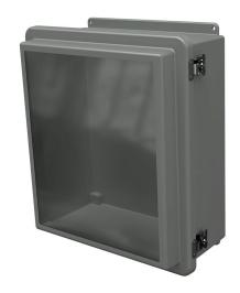
Stahlin RJW series enclosure, NEMA 1/3R/4X/6P/12,  $16 \times 14 \times 7$ in (HxWxD), wall mount, fiberglass reinforced polyester, gray, raised single-door, (2) twist-lock latches, SAR acrylic window.
