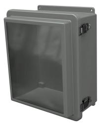
Stahlin RJW series enclosure, NEMA 1/3R/4X/6P/12, 14 x 12 x 7in (HxWxD), wall mount, fiberglass reinforced polyester, gray, raised single-door, (2) quick-release latches, padlock hasp and staple, SAR acrylic window.
