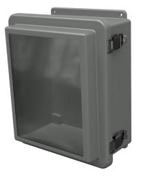
Stahlin RJW series enclosure, NEMA 1/3R/4X/6P/12, 12 x 10 x 6in (HxWxD), wall mount, fiberglass reinforced polyester, gray, raised single-door, (2) quick-release latches, padlock hasp and staple, SAR acrylic window.
