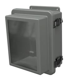
Stahlin RJW series enclosure, NEMA 1/3R/4X/6P/12, 10 x 8 x 6in (HxWxD), wall mount, fiberglass reinforced polyester, gray, raised single-door, (2) quick-release latches, padlock hasp and staple, SAR acrylic window.
