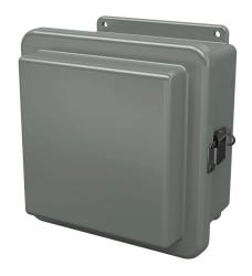
Stahlin RJ series enclosure, NEMA 1/3R/4X/6P/12, 8 x 8 x 6in (HxWxD), wall mount, fiberglass reinforced polyester, gray, raised single-door, (1) quick-release latch, padlock hasp and staple.
