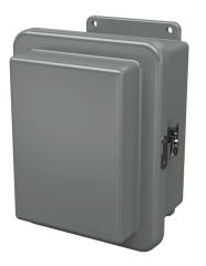
Stahlin RJ series enclosure, NEMA 1/3R/4X/6P/12, 8 x 6 x 6in (HxWxD), wall mount, fiberglass reinforced polyester, gray, raised single-door, (1) twist-lock latch.
