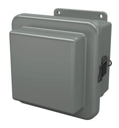
Stahlin RJ series enclosure, NEMA 1/3R/4X/6P/12, 6 x 6 x 6in (HxWxD), wall mount, fiberglass reinforced polyester, gray, raised single-door, (1) quick-release latch, padlock hasp and staple.
