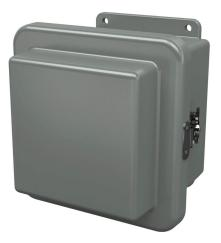
Stahlin RJ series enclosure, NEMA 1/3R/4X/6P/12, 6 x 6 x 6in (HxWxD), wall mount, fiberglass reinforced polyester, gray, raised single-door, (1) twist-lock latch.
