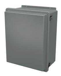
Stahlin RJ series enclosure, NEMA 1/3R/4X/6P/12,  $20 \times 16 \times 10$ in (HxWxD), wall mount, fiberglass reinforced polyester, gray, raised single-door, (2) twist-lock latches.
