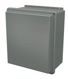
Stahlin RJ series enclosure, NEMA 1/3R/4X/6P/12, 18 x 16 x 10in (HxWxD), wall mount, fiberglass reinforced polyester, gray, raised hinged screw cover.
