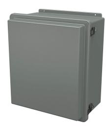
Stahlin RJ series enclosure, NEMA 1/3R/4X/6P/12, 18 x 16 x 10in (HxWxD), wall mount, fiberglass reinforced polyester, gray, raised single-door, (2) quick-release latches, padlock hasp and staple.
