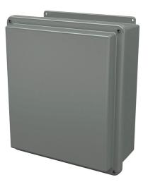
Stahlin RJ series enclosure, NEMA 1/3R/4X/6P/12, 16 x 14 x 7in (HxWxD), wall mount, fiberglass reinforced polyester, gray, raised screw cover.
