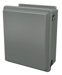
Stahlin RJ series enclosure, NEMA 1/3R/4X/6P/12,  $16 \times 14 \times 7$ in (HxWxD), wall mount, fiberglass reinforced polyester, gray, raised single-door, (2) twist-lock latches.
