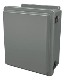
Stahlin RJ series enclosure, NEMA 1/3R/4X/6P/12,  $14 \times 12 \times 7in$  (HxWxD), wall mount, fiberglass reinforced polyester, gray, raised single-door, (2) quick-release latches, padlock hasp and staple.
