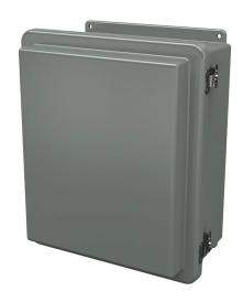
Stahlin RJ series enclosure, NEMA 1/3R/4X/6P/12,  $14 \times 12 \times 7$ in (HxWxD), wall mount, fiberglass reinforced polyester, gray, raised single-door, (2) twist-lock latches.
