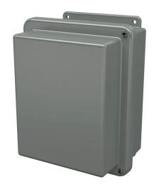
Stahlin RJ series enclosure, NEMA 1/3R/4X/6P/12, 10 x 8 x 6in (HxWxD), wall mount, fiberglass reinforced polyester, gray, raised hinged screw cover.
