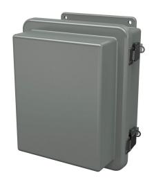
Stahlin RJ series enclosure, NEMA 1/3R/4X/6P/12, 10 x 8 x 6in (HxWxD), wall mount, fiberglass reinforced polyester, gray, raised single-door, (2) quick-release latches, padlock hasp and staple.
