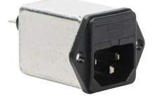
Roxburgh IEC inlet filter, 120/240 VAC, 1-phase, 6A, fused, screw mount, EMI/RFI filtering, 1-stage, general purpose, standard performance, 1/4in quick-disconnect.
