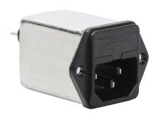
Roxburgh IEC inlet filter, 120/240 VAC, 1-phase, 2A, fused, screw mount, EMI/RFI filtering, 1-stage, general purpose, standard performance, 1/4in quick-disconnect.
