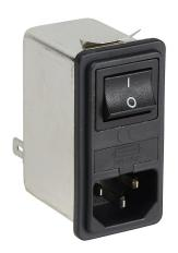
Roxburgh IEC inlet filter, 120/240 VAC, 1-phase, 6A, on/off switch, fused, snap-in mount, EMI/RFI filtering, 1-stage, general purpose, standard performance, 1/4in quick-disconnect.
