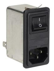
Roxburgh IEC inlet filter, 120/240 VAC, 1-phase, 4A, on/off switch, fused, snap-in mount, EMI/RFI filtering, 1-stage, general purpose, standard performance, 1/4in quick-disconnect.
