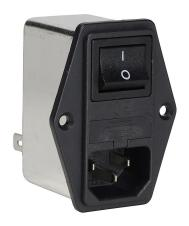
Roxburgh IEC inlet filter, 120/240 VAC, 1-phase, 6A, on/off switch, fused, screw mount, EMI/RFI filtering, 1-stage, general purpose, standard performance, 1/4in quick-disconnect.
