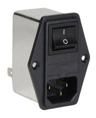
Roxburgh IEC inlet filter, 120/240 VAC, 1-phase, 2A, on/off switch, fused, screw mount, EMI/RFI filtering, 1-stage, general purpose, standard performance, 1/4in quick-disconnect.
