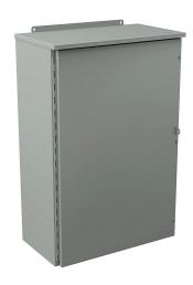
Wiegmann enclosure, NEMA 1/3R, 36 x 24 x 12in (HxWxD), wall mount, carbon steel, ANSI 61 gray, powder coat finish, singledoor, 1/4-turn flush-mounted latch, padlock hasp and staple.
