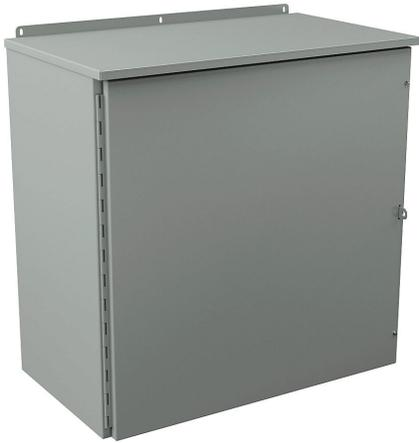
Wiegmann enclosure, NEMA 1/3R, 30 x 30 x 16in (HxWxD), wall mount, carbon steel, ANSI 61 gray, powder coat finish, single-door, 1/4-turn flush-mounted latch, padlock hasp and staple.
