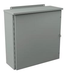
Wiegmann enclosure, NEMA 1/3R, 24 x 24 x 8in (HxWxD), wall mount, carbon steel, ANSI 61 gray, powder coat finish, single-door, 1/4-turn flush-mounted latch, padlock hasp and staple.
