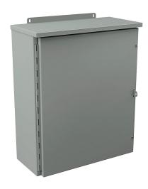
Wiegmann enclosure, NEMA 1/3R, 24 x 20 x 8in (HxWxD), wall mount, carbon steel, ANSI 61 gray, powder coat finish, single-door, 1/4-turn flush-mounted latch, padlock hasp and staple.
