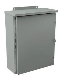
Wiegmann enclosure, NEMA 1/3R, 20 x 16 x 6in (HxWxD), wall mount, carbon steel, ANSI 61 gray, powder coat finish, single-door, 1/4-turn flush-mounted latch, padlock hasp and staple.
