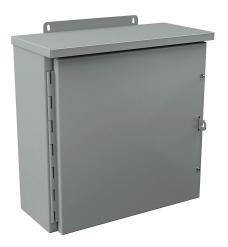
Wiegmann enclosure, NEMA 1/3R, 16 x 16 x 6in (HxWxD), wall mount, carbon steel, ANSI 61 gray, powder coat finish, single-door, 1/4-turn flush-mounted latch, padlock hasp and staple.
