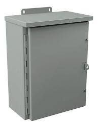
Wiegmann enclosure, NEMA 1/3R, 16 x 12 x 6in (HxWxD), wall mount, carbon steel, ANSI 61 gray, powder coat finish, single-door, 1/4-turn flush-mounted latch, padlock hasp and staple.
