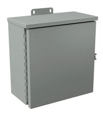
Wiegmann enclosure, NEMA 1/3R, 12 x 12 x 6in (HxWxD), wall mount, with knockouts, carbon steel, ANSI 61 gray, powder coat finish, single-door, (1) quick-release latch, padlock hasp and staple.
