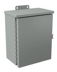
Wiegmann enclosure, NEMA 1/3R,  $12 \times 10 \times 6$  in (HxWxD), wall mount, with knockouts, carbon steel, ANSI 61 gray, powder coat finish, single-door, (1) quick-release latch, padlock hasp and staple.
