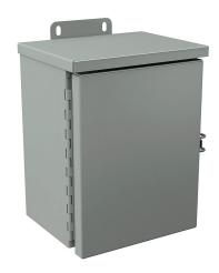
Wiegmann enclosure, NEMA 1/3R, 10 x 8 x 6in (HxWxD), wall mount, with knockouts, carbon steel, ANSI 61 gray, powder coat finish, single-door, (1) quick-release latch, padlock hasp and staple.
