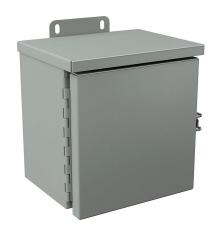
Wiegmann enclosure, NEMA 1/3R, 8 x 8 x 6in (HxWxD), wall mount, with knockouts, carbon steel, ANSI 61 gray, powder coat finish, single-door, (1) quick-release latch, padlock hasp and staple.
