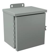
Wiegmann enclosure, NEMA 1/3R, 8 x 8 x 6in (HxWxD), wall mount, with knockouts, carbon steel, ANSI 61 gray, powder coat finish, single-door, (1) quick-release latch, padlock hasp and staple.
