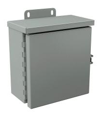
Wiegmann enclosure, NEMA 1/3R, 8 x 8 x 4in (HxWxD), wall mount, with knockouts, carbon steel, ANSI 61 gray, powder coat finish, single-door, (1) quick-release latch, padlock hasp and staple.
