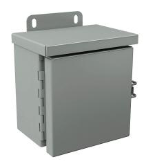
Wiegmann enclosure, NEMA 1/3R, 6 x 6 x 4in (HxWxD), wall mount, with knockouts, carbon steel, ANSI 61 gray, powder coat finish, single-door, (1) quick-release latch, padlock hasp and staple.
