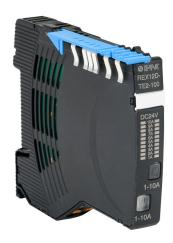
E-T-A REX series modular circuit protector, overcurrent protection, adjustable 1-10A, 24 VDC output, 2 independent channel(s), electronic, 35mm DIN rail mount.
