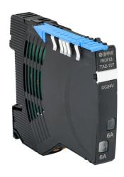
E-T-A REX series modular circuit protector, overcurrent protection, 6A, 24 VDC output, 2 independent channel(s), electronic, 35mm DIN rail mount.
