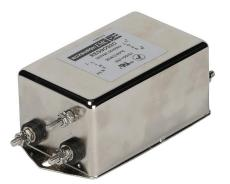
Roxburgh EMI input filter, 120/240 VAC, 1-phase, 20A, panel mount, EMI/RFI filtering, multi-stage, drive rated, very high performance, studs. For use with 1-phase AC drives.
