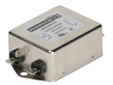
Roxburgh EMI input filter, 120/240 VAC, 1-phase, 3A, panel mount, EMI/RFI filtering, multi-stage, drive rated, very high performance, 1/4in quick-disconnect. For use with 1-phase AC drives.
