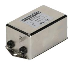
Roxburgh EMI input filter, 120/240 VAC, 1-phase, 6A, panel mount, EMI/RFI filtering, multi-stage, general purpose, high performance, 1/4in quick-disconnect.
