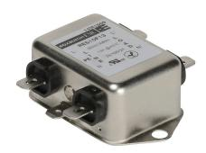
Roxburgh EMI input filter, 120/240 VAC, 1-phase, 13A, panel mount, EMI/RFI filtering, 1-stage, general purpose, standard performance, 1/4in quick-disconnect.
