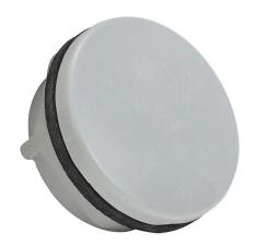
Stahlin hole plug, 1/2in conduit, fiberglass-reinforced plastic (FRP), closed-cell neoprene gasket. For use with non-metallic enclosures.
